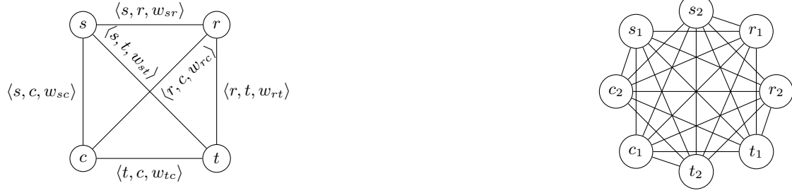
Fig. 2. Examples of models with 1 node (left) or 2 nodes (right) for each S , R , T and C , showing the different relations and the 4-partite structure (only nodes of the same type are not related).
